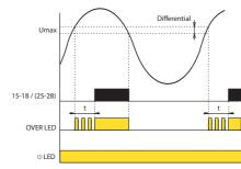
The time delay and differential trip levels help to prevent relay chatter as  $\frac{1}{2} \int_{\mathbb{R}^{n}} \frac{1}{2} \int_{\mathbb{R$ the monitored voltage level varies.
