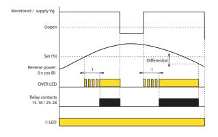
The time delay and differential trip levels help to prevent relay chatter as the monitored parameters fluctuate.
