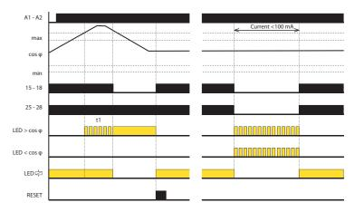
After powering on, the device sets the delay time t1 and yellow LED flashes. Both relays are switched on. The delay serves to eliminate a faulty state when starting the motor. After the time delay t1 begins monitoring COS  $\phi$  only.
