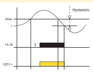
Monitoring relay PRI-52 serves for monitoring of current level in 1-phase AC circuits. Slight setting of release current level designates this relay for many various applications. Output relay is in normal status switched off. When set current level is overrun, relay get closed after preset delay. By return from error to normal status is used hysteresis.
