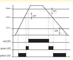
After connecting the supply voltage, the LED illuminates - the color corresponds to the voltage size of individual phases. If the phase voltage drops under 40 V (phase outage), the corresponding LED is not illuminated.
