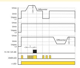
The time delay and differential trip levels help to prevent relay chatter as the monitored voltage level varies.
