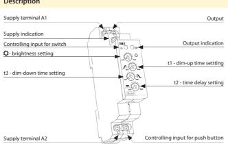
Recommendation for mounting: leave a gap of min. 0.5 module (approx. 9 mm) on side of the device to ensure better cooling of the device.
