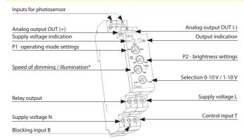
\* if the level of brightness on P2 is set on maximum the range is 24...120s
