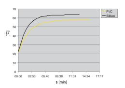
PVC -reaction to water temperature from 22.5 1 °C to 58 °C (from 72.5 °F to 136.4 °F).
