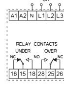
These units monitor a 3-phase 4-wire supply and operate relays if a phase-neutral voltage goes below or above set levels. Front panel controls allow selection of: 133
