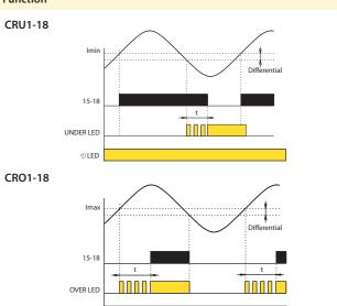
The time delay and differential trip levels help to prevent relay chatter as the monitored current level varies. As the relays have changeover contacts, the relay outputs can be inverted by wiring to the alternative terminals 15-16 or 25-26.
