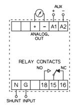
G - ground (grounding conductor)
