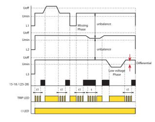
The time delay and differential trip levels help to prevent relay chatter as the monitored parameter fluctuates.
