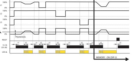
L1, L2, L3 - 3-phase voltage RESET - press of the button on frontal panel t1 - time pause, fixed
