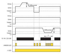
The time delay and differential trip levels help to prevent relay chatter as the monitored voltage level varies.
