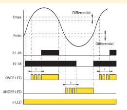
After the supply (monitored) voltage is connected, the green LED is on. If the value of the monitored frequency falls within the range between the two set levels Fmin - Fmax no red LED is on. The relay UNDER is triggered (contacts 15-16-18) and the relay OVER is disconnected (contacts 25-26-28).
