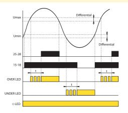
The time delay and differential trip levels help to prevent relay chatter as the monitored voltage level varies.
