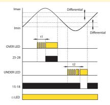
The time delay and differential trip levels help to prevent relay chatter as the monitored current level varies. As the relays have changeover contacts, the relay outputs can be inverted by wiring to the alternative terminals 15-16 or 25-26.
