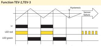
TEV-2 and TEV-3 are universal single thermostats for universal use. In case ambient temperature is higher than set temperature relay is open (function HEATING), for cooling function (opposite function) is possible to use NC contact of relay (V2).
