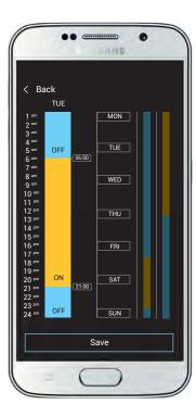
Through simple steps in the application you can set the desired on and off settings based on real time. You can copy this setting to other days, and altogether you can store up to 100 programs. The entire setup project can be saved to your smartphone and transferred to the next timer switch. The smartphone application serves not only to upload settings but also to download. The main benefit is speed and simplicity.
